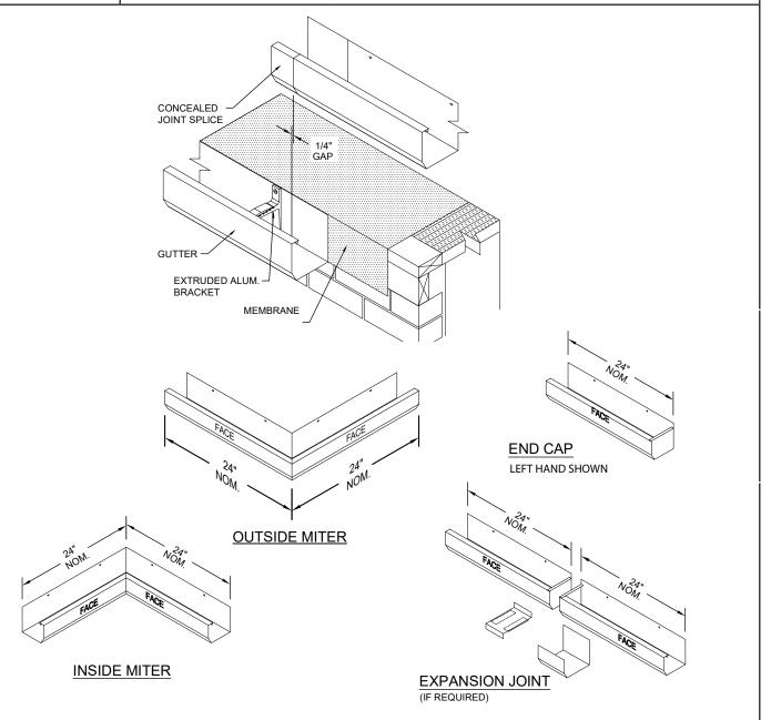
Standard gutter miter leg lengths are 24" Nominal Standard gutter miter angle is 90° For special miter requirements, attach sketches or consult manufacturer for assistance.
