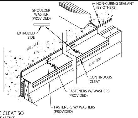
DO NOT OVERDRIVE THE SCREWS INTO THE CLEAT SO THAT THE SCREWS DO NOT RESTRICT MOVEMENT.
