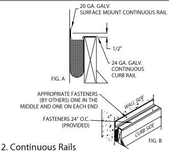
Fasten the 24 ga. galvanized continuous curb rail 24" O.C. to the top of the wood curb with provided fasteners (Fig. B). Fasten the 20 ga. galvanized surface mount continuous rail (edges facing out) to the wall (one fastener in the middle and one at each end) with an appropriate fastener (by others) suitable for substrate, with flatest head possible (see above). The center of the surface mount rail must be 1/2" above the top of the wood curb (Fig. A)
