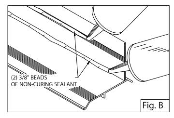
3. Miter & Scupper Anchor Bar (Preparation)
