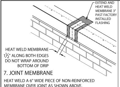
**HOT AIR WELD** ALONG LENGTH OF DRIP EDGE IF USING CARLSILE / VERSICO MEMBRANE APPLY CUT EDGE SEALANT ALONG EDGE IN AREAS OF PONDING WATER ONLY
