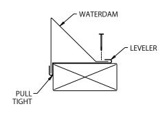
WATERDAM MUST BE PULLED TIGHT TO THE OUTSIDE FACE OF THE BUILDING BEFORE NAILING THE ROOF FLANGE.
