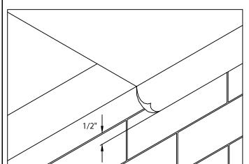
1. POSITION MEMBRANE OVER THE ROOF EDGE AND DOWN OUTSIDE FACE OF WALL, COVERING TREATED WOOD NAILER(S) COMPLETELY. ALLOW 1/3" EXCESS MEMBRANE.
