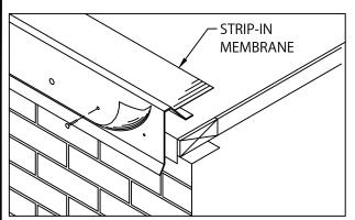
3. POSITION STRIP-IN MEMBRANE OVER AND DOWN WATERDAM FACE APPROXIMATELY 1" BELOW RAISED FASTENING HOLES (PROVIDED). TAKE CARE TO AVOID BRIDGING OF MEMBRANE. LOCATE AND NAIL MEMBRANE AT 12" O.C. THROUGH ALL RAISED HOLES ON OUTSIDE FACE USING PROVIDED FASTENERS.
