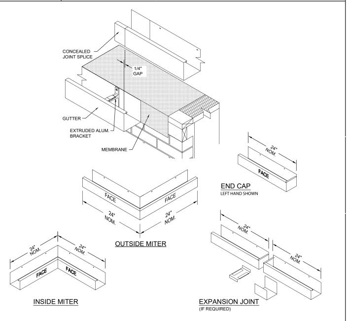
Standard gutter miter leg lengths are 24" Nominal Standard gutter miter angle is 90°
