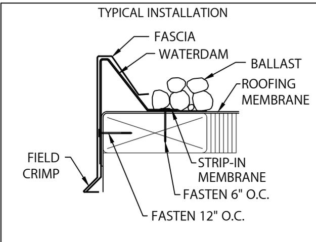
7. COMPLETE INSTALLATION BY PLACING BALLAST (IF REQUIRED), FOLLOWING ROOF MEMBRANE MANUFACTURERS' RECOMMENDATIONS.
