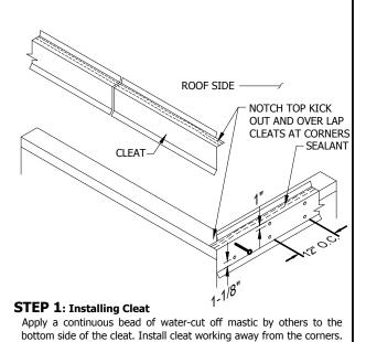
Attach the cleat using 1-1/2" SS ring shank nails at the locations shown above at 12" O.C. The lower row of fasteners are only
