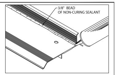
2. Miter & Scupper Anchor Bar (Preparation) Lay miters and scuppers on deck with outside face down. Be sure aluminum anchor bar is clean and free of dirt or dust. Apply a heavy 3/8" bead of non-curing sealant to the right angle inter-section of the deck flange and back of anchor bar as shown. Application of sealant is required along the full length of each miter anchor bar.
