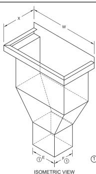
(1) "E" & "F" are sized 1/4" less than the size of the downspout to be used.
