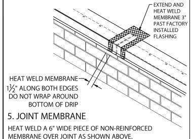
**HOT AIR WELD** ALONG LENGTH OF DRIP EDGE IF USING CARLSILE / VERSICO MEMBRANE APPLY CUT EDGE **SEALANT ALONG EDGE** IN AREAS OF PONDING WATER ONLY
