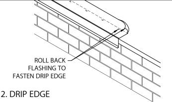
PLACE DRIP EDGE ON WALL. ROLL BACK FLASHING TO EXPOSE FASTENING SLOTS AND FASTEN THRU PRE-SLOTTED HOLES 6" WITH PROVIDED FASTENERS.
