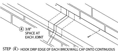
STEP 4- HOOK DRIP EDGE OF EACH BRICK/WALL CAP ONTO CONTINUOUS CLEAT, ROTATE INTO PLACE, AND FASTEN WITH APPROPRIATE FASTENERS. CONTINUE BY INSTALLING BRICK/WALL CAP SECTIONS AND SPLICE PLATES, ALLOWING A 3/8" SPACE AS SHOWN. FIELD CUT AS NECESSARY.
