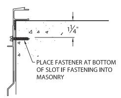
PLACE FASTENER AT BOTTOM OF SLOT IF FASTENING INTO ELIMINAILER.
