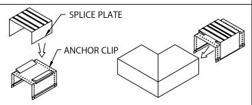
STEP 2 - MITER SPLICE PLATES & ANCHOR CLIPS POSITION THE SPLICE PLATE IN THE CENTER OF THE ANCHOR CLIP. INSTALL THE SPLICE PLATE AND ANCHOR CLIP ASSEMBLY INTO EACH END OF THE CORNER AS SHOWN
