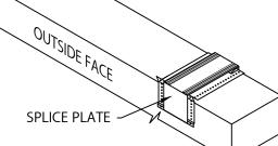
STEP 8 - SPLICE PLATES PLACE SPLICE PLATE ONTO ANCHOR CLIPS AT SPLICE JOINTS, 12'-0" O.C. NOTE: REMOVE RELEASE PAPER FROM SEALANT STRIPS. STEP 7 - ANCHOR CLIPS
