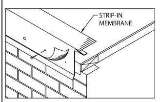
3. POSITION STRIP-IN MEMBRANE OVER AND DOWN WATERDAM FACE APPROXIMATELY 1" BELOW RAISED FASTENING HOLES (PROVIDED). TAKE CARE TO AVOID BRIDGING OF MEMBRANE. LOCATE AND NAIL MEMBRANE AT 12" O.C. THROUGH ALL RAISED HOLES ON OUTSIDE FACE USING PROVIDED FASTENERS.
