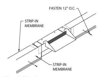
STEP 3 - WATERDAM POSITION STRIP-IN MEMBRANE OVER AND DOWN WATERDAM FACE APPROXIMATELY 1" BELOW RAISED FASTENING HOLES. TAKE CARE TO AVOID BRIDGING OF MEMBRANE. LOCATE AND FASTEN MEMBRANE AT 12" O.C. THROUGH ALL RAISED HOLES ON OUTSIDE FACE USING PROVIDED FASTENERS.
