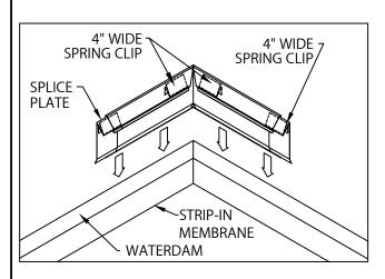
4. INSTALL MITER COVERS FIRST. INSERT ONE SPLICE PLATE AND ONE 4" WIDE SPRING CLIP INTO EACH END OF MITER COVER, (SEE DETAIL ON PAGE 3 FOR PROPER SPRING INSTALLATION). PLACE TWO 4" WIDE SPRING CLIPS INTO CORNERS OF MITER AS SHOWN. INSTALL MITER COVERS BY PUSHING DOWNWARD UNTIL COVER IS ENGAGED ALONG ENTIRE MITER.
