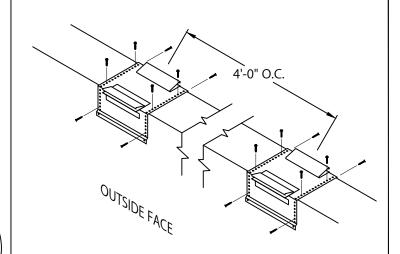
STEP 7 - ANCHOR CLIPS LOCATE AND FASTEN GALVANIZED ANCHOR CLIPS TO WALL AT 4'-0" CENTERS WITH PROVIDED FASTENERS FOR SUBSTRATE (SEE DETAIL A).
