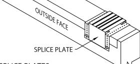
**STEP 8 - SPLICE PLATES** PLACE SPLICE PLATE ONTO ANCHOR CLIPS AT SPLICE JOINTS, 12'-0" O.C. NOTE: REMOVE RELEASE PAPER FROM SEALANT STRIPS.
