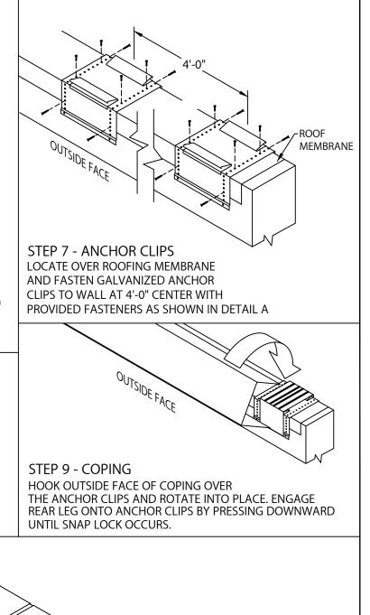
OUTSIDE FACE 3/8" **STEP 10 - COMPLETION** SPACE CONTINUE INSTALLING COPING WITH A 3/8" SPACE AT SPLICE JOINTS TO ALLOW FOR THERMAL EXPANSION. FIELD CUT WHERE NECESSARY USING FINE TOOTH HACKSAW OR SNIPS. NOTE: REMOVE PROTECTIVE FILM IMMEDIATELY. DATE: 06/17/22 Customer Service DRN BY: MLM 800-558-2162 CKD BY: MM
