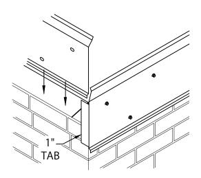
STEP 3 - RAIL MITER PREPARATION SEE PAGE 5 FOR MITER PREPARATION. FASTEN MITER BASE RAIL TO NAILER(S) THROUGH BASE RAIL SLOTS WITH PROVIDED FASTENERS.
