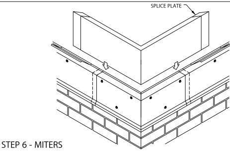
PLACE SPLICE PLATE INTO EACH END OF MITER COVER. SIMPLY POSITION THE COVER ABOVE THE RAIL AND WITH PALM OF HAND APPLY SLIGHT PRESSURE DOWNWARD UNTIL ENGAGED TO THE BOTTOM OF BASE RAIL. IF MITERS ARE NOT SUPPLIED, SEE PAGE 6 FOR FABRICATION INSTRUCTIONS.
