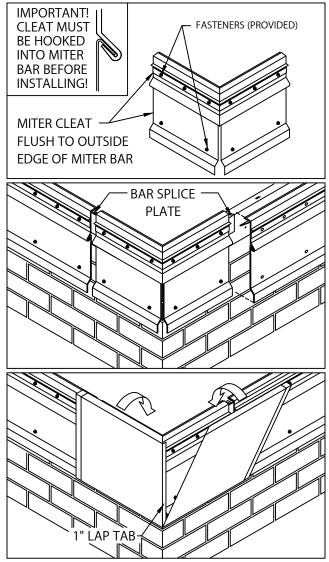
5. MITER BAR & MITER CLEAT INSTALLATION HOOK MITER CLEAT PIECES TO MITER BAR. FLUSH ENDS OF MITER CLEAT PIECE AND MITER BAR. INSTALL MITER ASSEMBLY WITH ONE ANCHOR BAR SPLICE PLATE UNDER EACH END OF MITER BAR. FASTEN THE MITER BAR USING PROVIDED FASTENERS AND DRIVE BITS. NEXT LOCATE AND INSTALL THE SCUPPERS WITH FASTENERS AND SPLICE PLATES.
