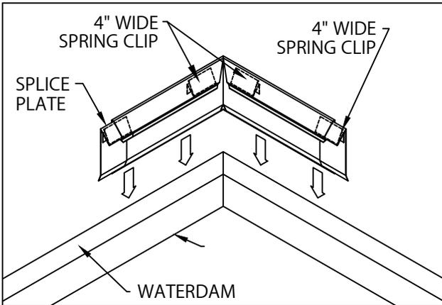
4. INSTALL MITER COVERS FIRST. INSERT ONE SPLICE PLATE AND ONE 4" WIDE SPRING CLIP INTO EACH END OF MITER COVER, (SEE DETAIL ON PAGE 3 FOR PROPER SPRING INSTALLATION). PLACE TWO 4" WIDE SPRING CLIPS INTO CORNERS OF MITER AS SHOWN. INSTALL MITER COVERS BY PUSHING DOWNWARD UNTIL COVER IS ENGAGED ALONG ENTIRE MITER.
