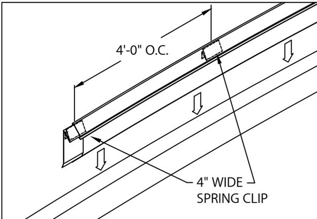
2. INSTALL 12'-0" FASCIA COVER SECTIONS. INSERT ONE SPLICE PLATE AND ONE 4" WIDE SPRING CLIP UNDER FAR END OF FASCIA COVER. PLACE 4" WIDE SPRING CLIPS INTO COVER AT 4'-0" O.C. INSTALL COVER BY PUSHING DOWNWARD UNTIL FASCIA COVER IS ENGAGED TO WATERDAM ALONG ENTIRE LENGTH. CONTINUE TO INSTALL FASCIA COVERS, LEAVING A 3/8" SPACE BETWEEN COVERS. FIELD CUT WHERE NECESSARY USING FINE TOOTH HACKSAW.
