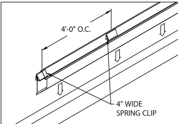
5. INSTALL 12'-0" FASCIA COVER SECTIONS. INSERT ONE SPLICE PLATE AND ONE 4" WIDE SPRING CLIP UNDER FAR END OF FASCIA COVER. PLACE 4" WIDE SPRING CLIPS INTO COVER AT 4'-0" O.C. INSTALL COVER BY PUSHING DOWNWARD UNTIL FASCIA COVER IS ENGAGED TO WATERDAM ALONG ENTIRE LENGTH. CONTINUE TO INSTALL FASCIA COVERS, LEAVING A 3/8" SPACE BETWEEN COVERS. FIELD CUT WHERE NECESSARY USING FINE TOOTH HACKSAW.
