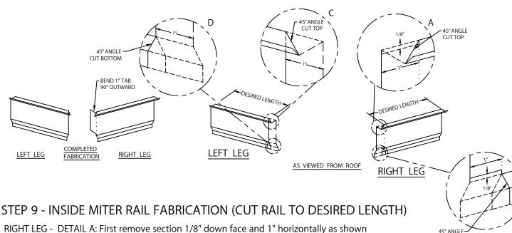
RIGHT LEG - DETAIL A: First remove section 1/8" down face and 1" horizontally as shown to create tab. Trim top flange back at a 45° angle. DETAIL B: Cut off bottom face 1/8" as shown and continue cut at a 45° through area shown on bottom flange. Bend tab inwards 90°. LEFT LEG - DETAIL C: Cut top flange at a 45° angle. Continue down face. DETAIL D: Cut bottom
