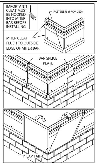
5. MITER BAR & MITER CLEAT INSTALLATION HOOK MITER CLEAT PIECES TO MITER BAR. FLUSH ENDS OF MITER CLEAT PIECE AND MITER BAR. INSTALL MITER ASSEMBLY WITH ONE ANCHOR BAR SPLICE PLATE UNDER EACH END OF MITER BAR. FASTEN THE MITER BAR USING FASTENERS AND DRIVE BITS PROVIDED. NEXT LOCATE AND INSTALL THE SPILLOUTS AND SCUPPERS WITH FASTENERS AND SPLICE PLATES.
