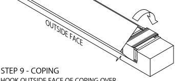
HOOK OUTSIDE FACE OF COPING OVER THE ANCHOR CLIPS AND ROTATE INTO PLACE. ENGAGE REAR LEG ONTO ANCHOR CLIPS BY PRESSING DOWNWARD UNTIL SNAP LOCK OCCURS.
