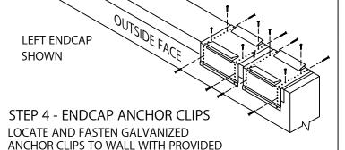
FASTENERS FOR SUBSTRATE (SEE DETAIL A).
