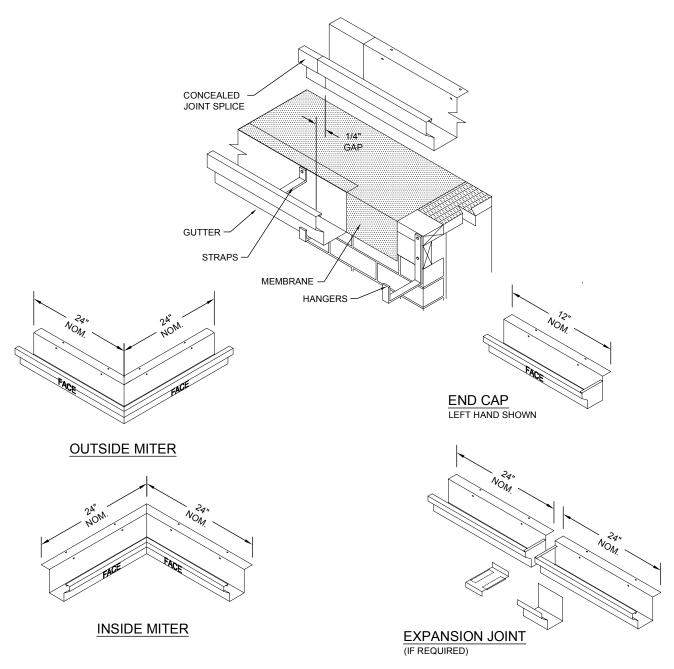
Standard gutter miter leg lengths are 24" Nominal Standard gutter miter angle is 90° For special miter requirements, attach sketches or consult manufacturer for assistance.
