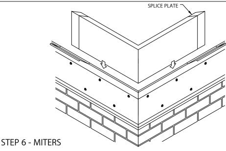
PLACE SPLICE PLATE INTO EACH END OF MITER COVER. SIMPLY POSITION THE COVER ABOVE THE RAIL AND WITH PALM OF HAND APPLY SLIGHT PRESSURE DOWNWARD UNTIL ENGAGED TO THE BOTTOM OF BASE RAIL.
