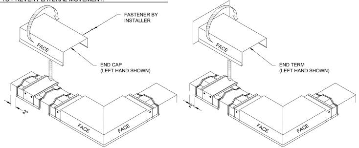
NOTE: ALL MITERS, END CONDITIONS, AND ACCESSORY CONDITIONS SHOULD BE INSTALLED PRIOR TO STRAIGHT SECTIONS
