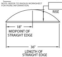
NOTE: CHECK MEASUREMENTS ALONG ENTIRE RADIUS **DETAIL A**
