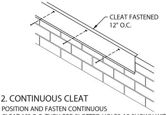
CLEAT 12" O.C. THRU PRE-SLOTTED HOLES AS SHOWN WITH PROVIDED FASTENERS. LAP CLEAT 1" AT JOINTS.
