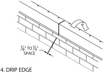
CONTINUE INSTALLING 12'-0" LENGTHS OF DRIP EDGE. LEAVE A  $\frac{1}{8}$ " TO  $\frac{1}{4}$ " SPACE BETWEEN PIECES.
