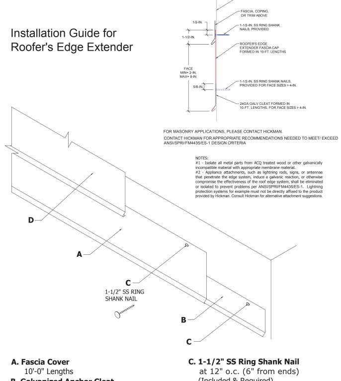
**B. Galvanized Anchor Cleat** for face size > 4" 10'-0" Lengths
