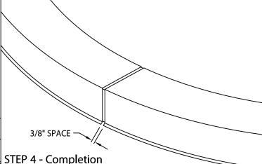
Continue installing coping with a 3/8" space at splice joints to allow for thermal expansion. Field cut where necessary using a fine tooth hacksaw or snips. NOTE: REMOVE PROTECTIVE FILM IMMEDIATELY.
