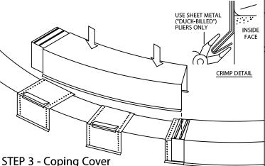
Remove release paper from right two factory applied sealant strips on the splice plate in the coping section. Install 4'-0" radius coping sections from left to right. Place coping into position and press downward until snap-lock occurs. Field crimp inside drip at all anchor clips.
