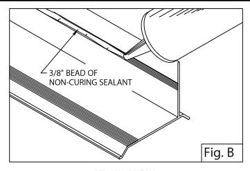
3. Miter & Scupper Anchor Bar (Preparation)
