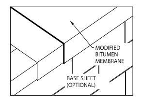
NOTE: Some manufacturers may require a "sacrificial" flashing strip. (Refer to drawing 2A & 2B) Please check with membrane manufacturer prior to installation.
