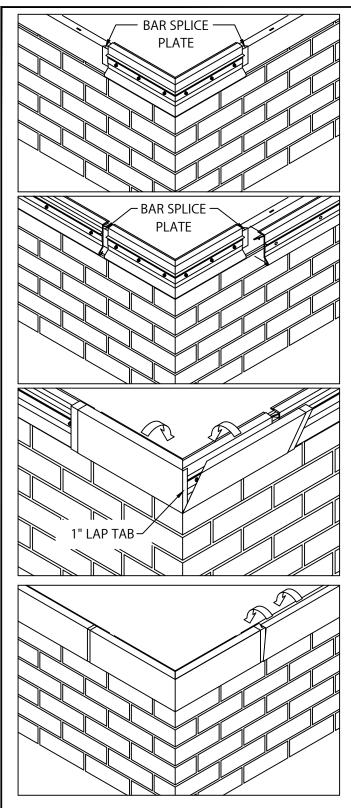
**3. MITER BAR INSTALLATION** INSTALL MITER ANCHOR BAR WITH ONE ANCHOR BAR SPLICE PLATE UNDER EACH END OF MITER BAR. FASTEN THE MITER BAR
