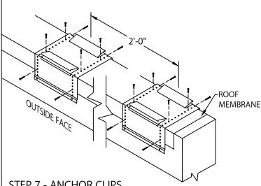
STEP 7 - ANCHOR CLIPS LOCATE OVER ROOFING MEMBRANE AND FASTEN GALVANIZED ANCHOR CLIPS TO WALL AT 2'-0" CENTER WITH PROVIDED FASTENERS AS SHOWN IN DETAIL A
