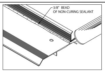
2. Miter & Scupper Anchor Bar (Preparation) Lay miters and scuppers on deck with outside face down. Be sure aluminum anchor bar is clean and free of dirt or dust. Apply a heavy 3/8" bead of non-curing sealant to the right angle inter-section of the deck flange and back of anchor bar as shown. Application of sealant is required along the full length of each miter anchor bar.
