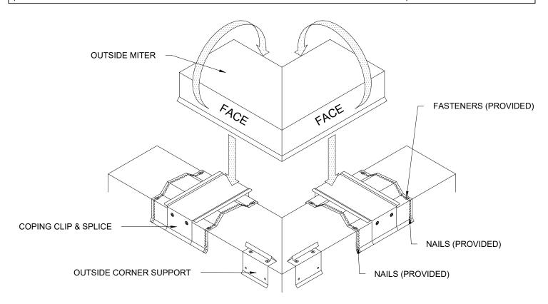
STEP 5: PLACE CLIPS AT END LOCATIONS SHOWN BELOW AND LOCATE END CAPS/END TERMS AND HOOK ON FRONT OF CLIP, ROTATE BACKWARD AND PRESS DOWNWARD TO ENGAGE ONTO CLIP. \*SECURE ENDCAP TO CLIP USING POP-RIVET OR SCREW (BY INSTALLER) TO PREVENT LATERAL MOVEMENT.
