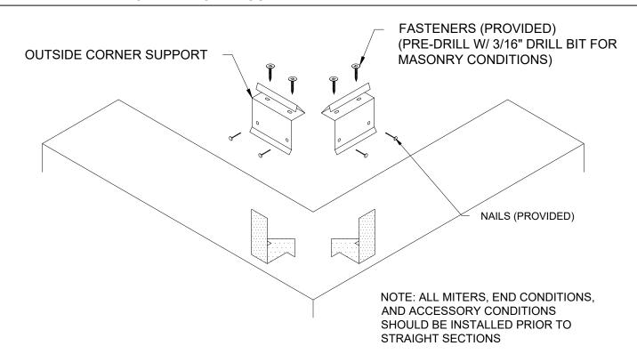
STEP 2: ALIGN CENTER OF EACH CLIP FROM THE CORNER SUCH THAT THE MITER LEG SITS HALF-WAY OVER EACH CLIP AS SEEN IN STEPS 3 & 4 (PAGE 4)
