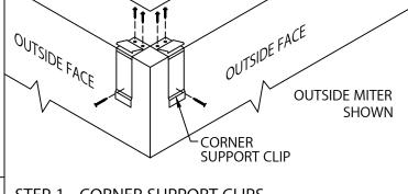
STEP 1 - CORNER SUPPORT CLIPS LOCATE AND FASTEN GALVANIZED CORNER SUPPORT CLIPS TO THE WALL.
