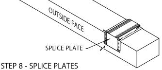
PLACE SPLICE PLATE ONTO ANCHOR CLIPS AT SPLICE JOINTS, 12'-0" O.C.
