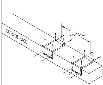
STEP 7 - ANCHOR CLIPS LOCATE OVER MEMBRANE AND FASTEN GALVANIZED ANCHOR CLIPS TO WALL AT 3'-0" CENTER WITH PROVIDED FASTENERS AS SHOWN IN DETAIL A.
