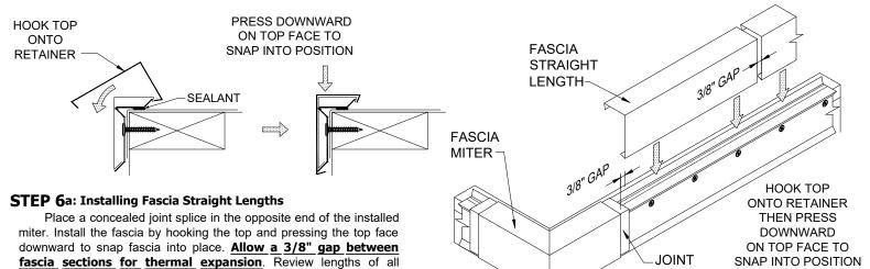
straight pieces prior to cutting to avoid creating relatively short sections of fascia adjacent to full length sections. (DO NOT HOOK THE BOTTOM OF THE SPLICE ONTO THE RETAINER) Note: There must be a splice at every joint.
