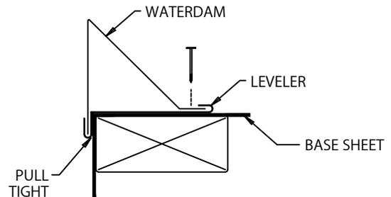
WATERDAM MUST BE PULLED TIGHT TO THE OUTSIDE FACE OF THE BUILDING BEFORE NAILING THE ROOF FLANGE.
