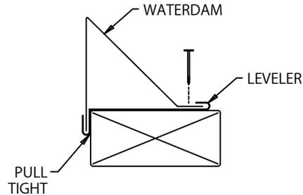
WATERDAM MUST BE PULLED TIGHT TO THE OUTSIDE FACE OF THE BUILDING BEFORE NAILING THE ROOF FLANGE.
