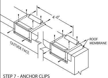
LOCATE OVER ROOFING MEMBRANE AND FASTEN GALVANIZED ANCHOR CLIPS TO WALL AT 4'-0" CENTER WITH PROVIDED FASTENERS AS SHOWN IN DETAIL A
