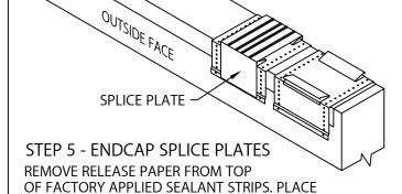
SPLICE PLATE ONTO SECOND ANCHOR CLIP AS SHOWN.
