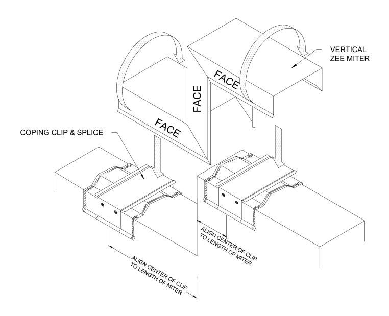
NOTE: ALL MITERS, END CONDITIONS, AND ACCESSORY CONDITIONS SHOULD BE INSTALLED PRIOR TO STRAIGHT SECTIONS
