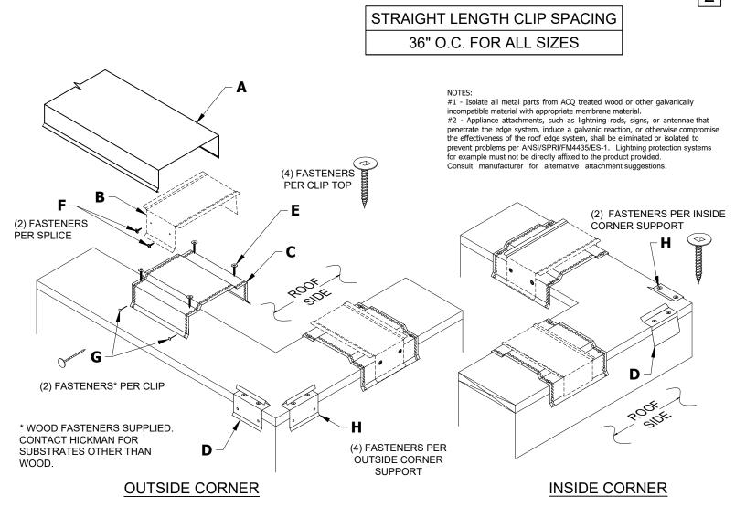
NOTE: ALL MITERS, END CONDITIONS, AND ACCESSORY CONDITIONS SHOULD BE INSTALLED PRIOR TO STRAIGHT SECTIONS
