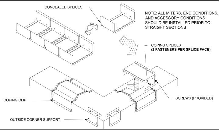
STEP 4: LOCATE MITER AND PLACE ONE LEG OVER THE CORNER SUPPORT AND CLIP, ROTATE BACKWARD AND PRESS DOWNWARD ON CAP TO ENGAGE ONTO CLIP, THEN REPEAT ON ADJACENT LEG OF MITER. (INSIDE MITER IS INSTALLED IN THE SAME MANNER USING INSIDE CORNER SUPPORTS).
