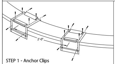
Locate and fasten anchor clips at 2'-0" O.C. with provided fasteners for substrate (see detail A).
