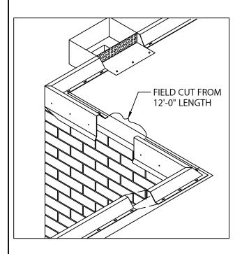
2. LOCATE AND INSTALL MITERS, NAILING THROUGH PRE-SLOTTED FASTENING HOLES ON TOP FLANGE ONLY. DETERMINE AND IDENTIFY LOCATION OF SCUPPERS. LEAVE GAP OF 14 1/2" INCHES FOR SCUPPER LOCATIONS. NEXT LOCATE AND INSTALL SCUPPERS. SEE PAGES 4 AND 5 FOR DETAILED INSTRUCTIONS ON INSTALLING SCUPPERS, THEN INSTALL THE 12'-0" SECTIONS OF WATERDAM FROM RIGHT TO LEFT (AS SEEN FROM ROOF TOP) BY NAILING THROUGH SLOTTED HOLES PROVIDED PER JOB REQUIREMENTS. FIELD CUT SECTIONS AS NECESSARY. LAP WATERDAM JOINTS 1".
