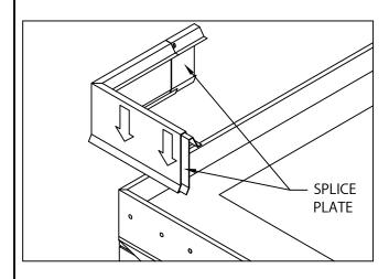
4. INSTALL MITER COVERS FIRST. INSERT ONE SPLICE PLATE UNDER EACH END OF MITER COVER. ALLOW 3/8" SPACE BETWEEN ENDS OF ADJOINING FASCIA PANELS. INSTALL MITER COVERS BY PUSHING DOWNWARD UNTIL COVER IS ENGAGED ALONG ENTIRE MITER. CRIMP ENTIRE DRIP EDGE OF EACH MITER COVER AS SHOWN IN STEP #6.
