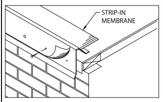
3. POSITION STRIP-IN MEMBRANE OVER AND DOWN WATERDAM FACE APPROXIMATELY 1" BELOW RAISED FASTENING HOLES (PROVIDED).
