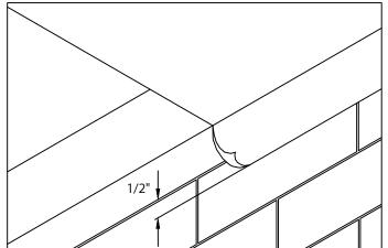
1. POSITION MEMBRANE OVER THE ROOF EDGE AND DOWN OUTSIDE FACE OF WALL, COVERING TREATED WOOD NAILER(S) COMPLETELY. ALLOW 1/2" EXCESS MEMBRANE.
